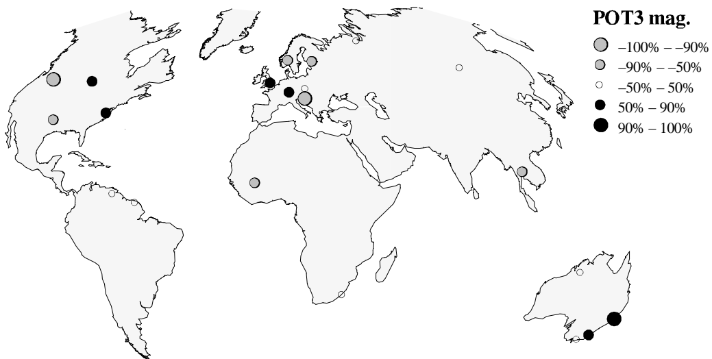
Figure 4. As in Figure 2, but for trends in the peak-over-threshold magnitude series, with on average 3 daily mean river flow peaks per year selected.
