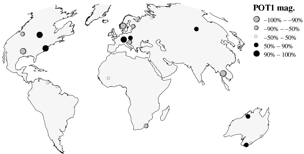
Figure 3. As in Figure 2, but for trends in the peak-over-threshold magnitude series, with on average 1 daily mean river flow peak per year selected.
